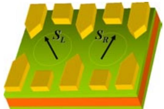
**Figure 1:** A double quantum dot. Top gates confine electrons in the two-dimensional electron gas to the circular regions. A negative voltage on the backgate depletes the dots until they contain a single electron with a spin  $\frac{1}{2}$  described by  $\mathbf{S}_L$  and  $\mathbf{S}_R$ . The corresponding  $|\uparrow\rangle$  and  $|\downarrow\rangle$  states form the qubit basis.
