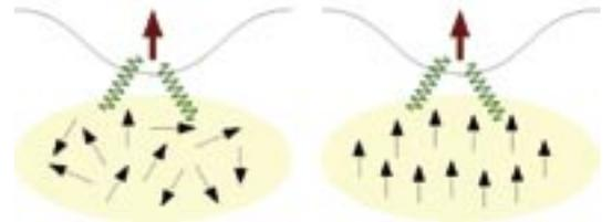
**Figure 2:** Illustration of the hyperfine interaction of the electron spin in the quantum dot with nearby nuclear spins. Disorder of the nuclear spins is an important source of decoherence (left). It can be largely reduced by polarization of the nuclear spins (right) as, for instance, achieved through a ferromagnetic phase transition triggered by many-body interactions.
