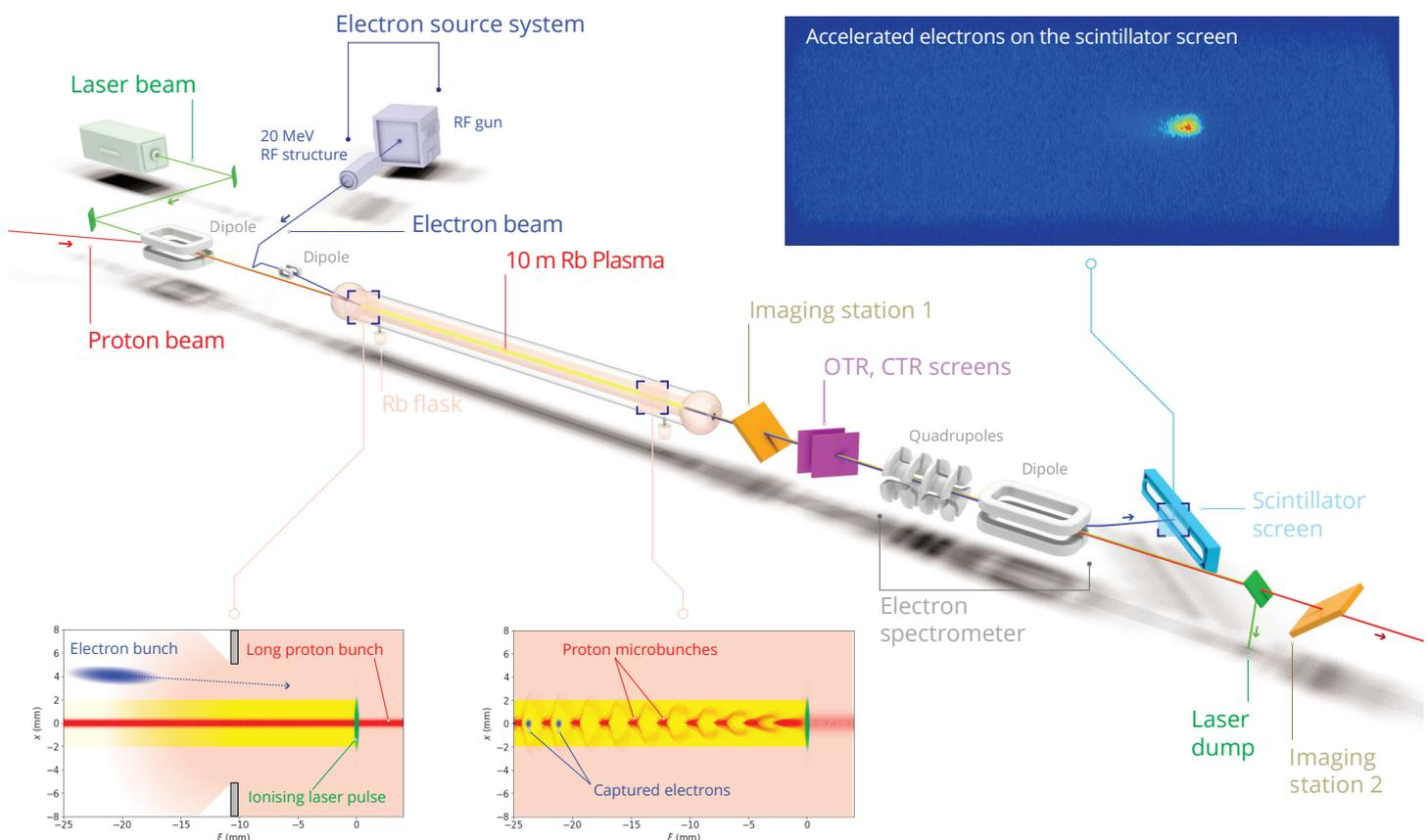
Fig. 1: Schematic layout of the AWAKE experiment.
